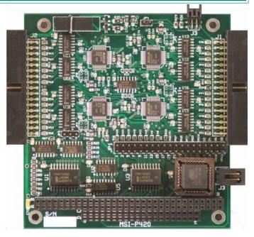
ranges with capacities of 8, 16, 24 or 32 channels which operate from a single +5V supply with a non-linearity of  $\pm 1/2$  LSB. The inputs are overvoltage tolerant to  $\pm 15V$ . A block diagram of the card is shown in Fig. 1.
